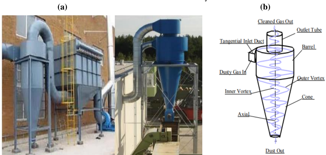
Figure 1: Pictorial and Schematic flow diagrams of a cyclone
